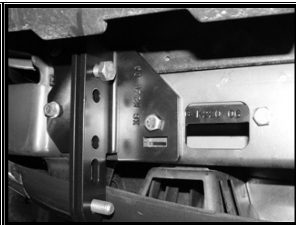
Photo 2. Passenger side view showing location of inside mounting bracket and Backing plate.
