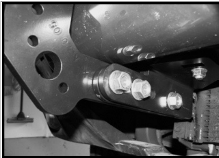
Photo 3. Passenger side view showing location of Light Tab Bracket relative to where the Outside and Inside Mounting Brackets meet.
