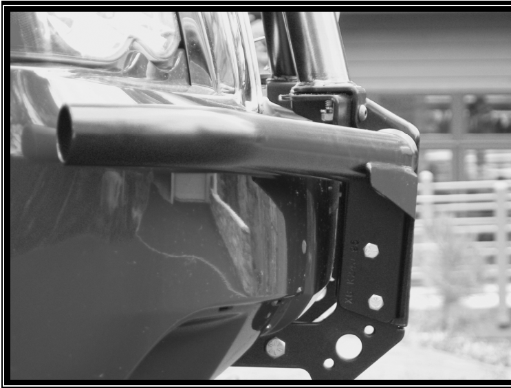
Photo 4. Passenger side view showing completed installation and proper alignment of Brush Rail (note the slight forward tilt of the top of the Light Tab Brackets).
