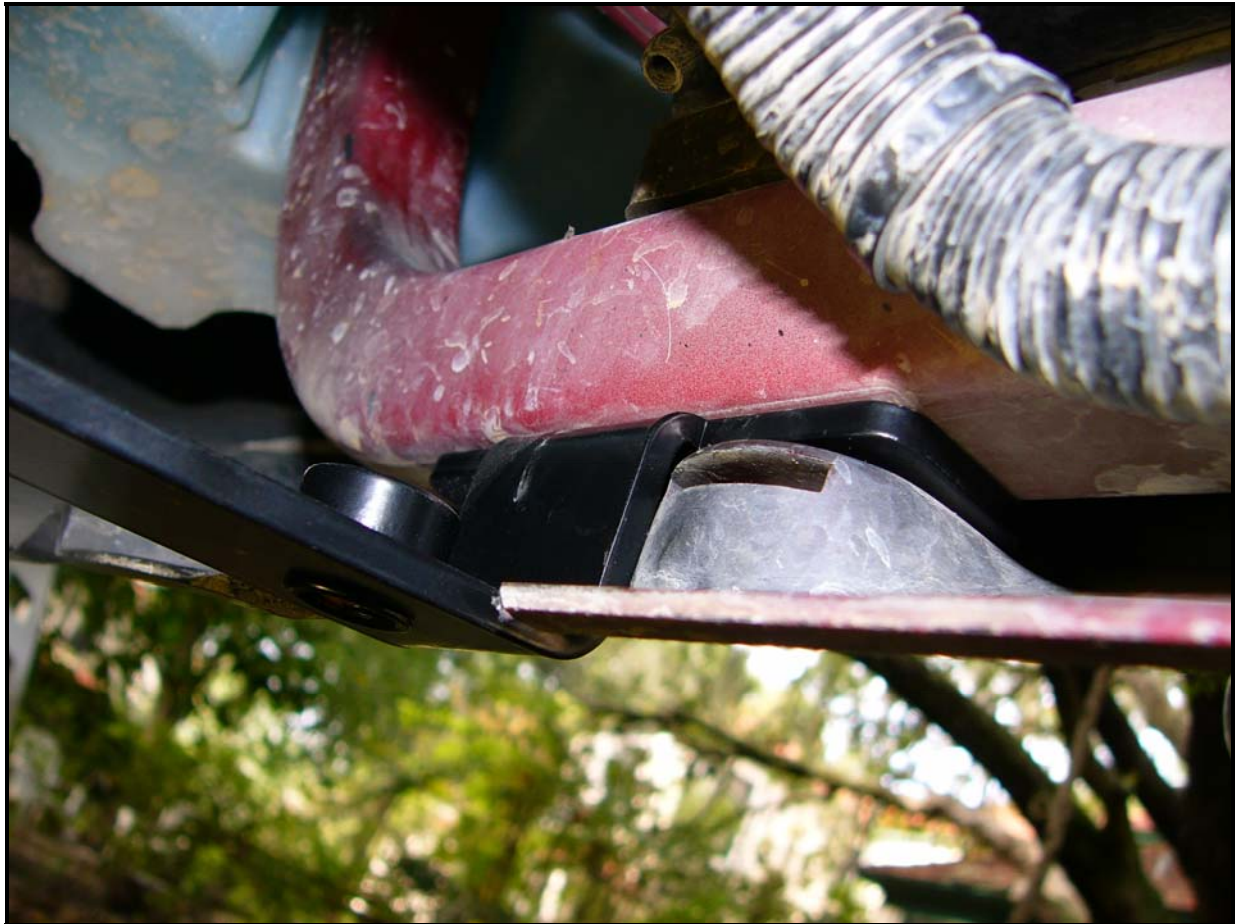
Photo 4. Driver-side Front Guard mounting bracket properly seated against crossmember through slot cut in fascia. Note tightness against recess in fascia.
