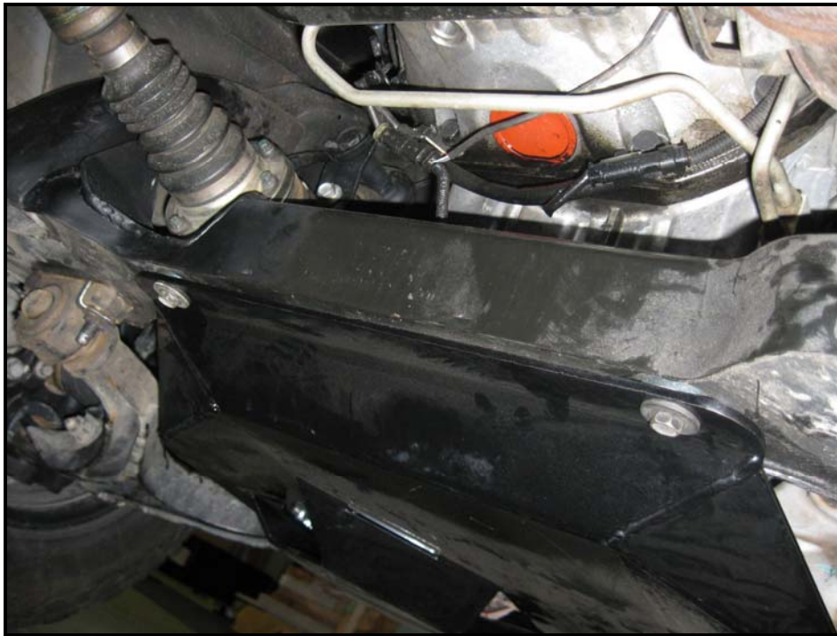
Figure 1 , showing two bolts in front crossmember.
