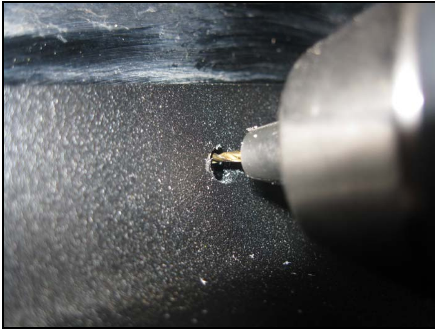
Figure 1. Drilling holes for the upper flange at the top of the hole in the Side Guard.
