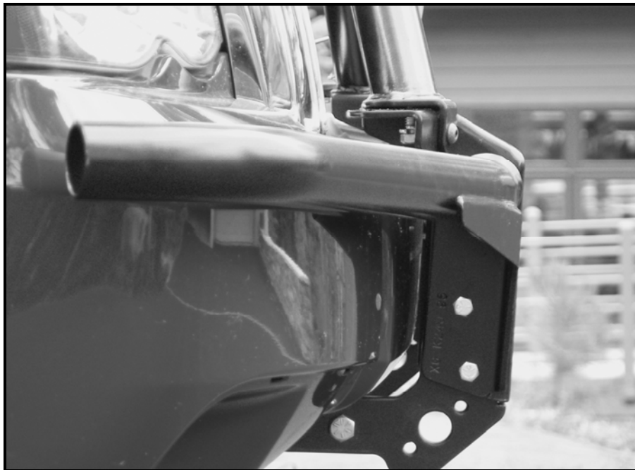
Photo 4. Passenger-side view showing completed installation and proper alignment of optional Matrix Brush Rail (note the slight forward tilt of the top of the light tab brackets).
