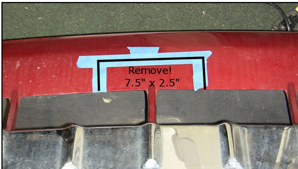
Commander fascia showing necessary alterations to fit optional receiver mount.
